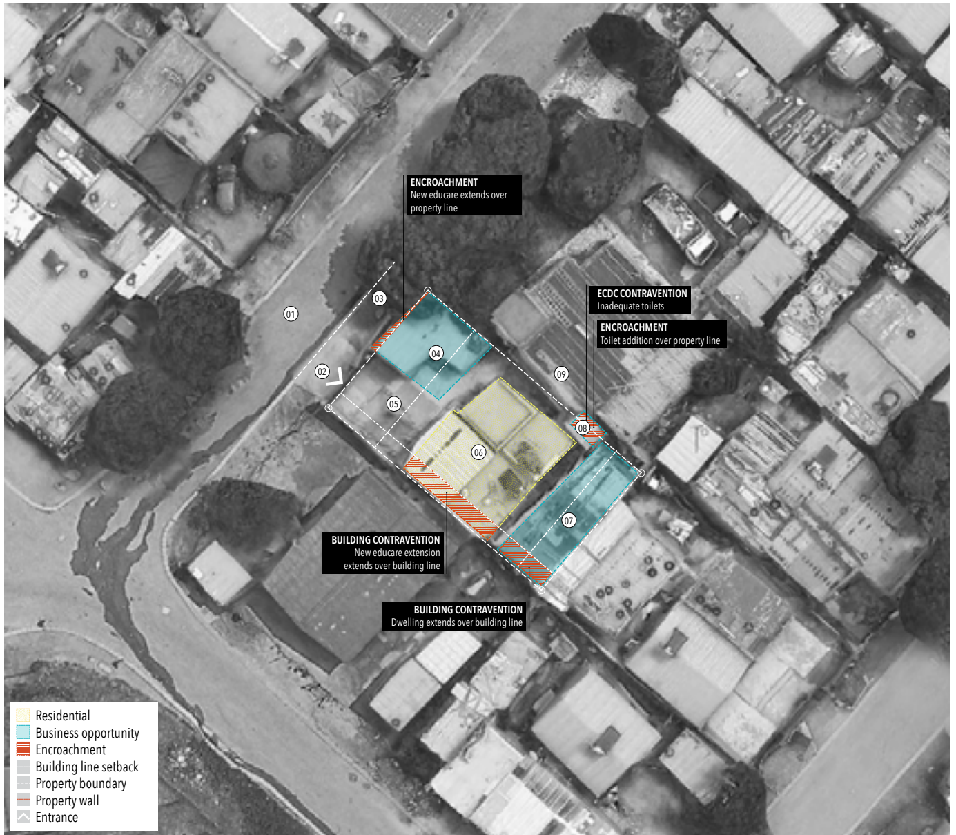
SITUATION PLAN: Aerial image illustrating the existing property uses relative to regulatory frameworks.
